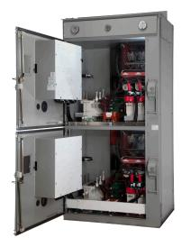
Benshaw's MVDH Two-High Solid State Starters provide separate medium and low voltage sections for each starter. Both sections include a complete starter - load break disconnect switch, Class R rated fuses, inline and bypass contactors and power stacks, to allow complete independent control of two motors.
