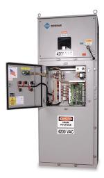
Benshaw's legacy MVRXE Solid State Soft Starter is a microprocessor-controlled, reduced voltage soft starter for three phase induction motors. MVRXE Series soft starters from Benshaw are designed for severe duty applications and offer a closed-loop current ramp for smooth, stepless motor acceleration.
