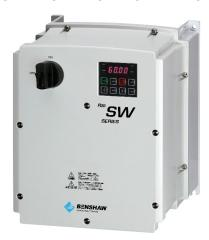
Benshaw SW Series NEMA 4X Washdown Drives are heavy duty rated for applications from 0.5-30HP. Designed for high pressure washdown, all SW Series drives feature a rugged UL Type 4X (IP66) indoor rated polycarbonate enclosure that exceeds NEMA 1, 12, 4 and 4X standard. A convenient built-in power disconnect switch, 4 digit- 7 segment display an optional remote keypad make it easy to control.
