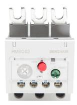
RMSO/SPO Series Overload Relays are bimetallic-style relays designed to protect AC-3 circuits (up to 150A @ 690V) and motors against overloads, phase failure, long starting times and stalling of the motor. RMSO and SPO Series overload relays can be integrally mounted to Benshaw RC and RSC contactors for thermal overload protection.
