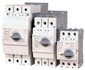
RMXP Series manual starters offer efficient motor starting functionality in a compact design. Protection functions include circuit, motor, starter and phase failure protection. They couple directly to RC Series contactors for a complete electro-mechanical combination starter.
