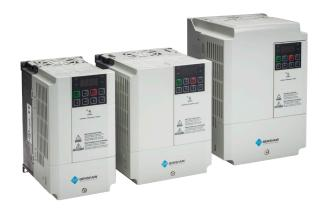
Benshaw S Series Variable Frequency Micro Drives provide a rugged, compact, economical chassis drive solution for low horsepower applications. Each drive in the series offers quick setup and preconfigured settings for common VFD applications, and a flexible, programmable I/O for more demanding applications or complex control strategies. Dual rated for both variable torque (120%) and constant torque (150%).
