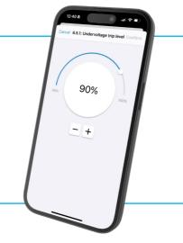
Easily adjust your starter's parameter values, offering a faster, more convenient alternative to the physical HMI. Backup, restore, or transfer parameter settings between starters with simple import/export functionality. Create custom text labels for specific parameters, like personalized trip names for configurable I/O.
