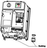
3 Connect the power cables to the power terminals and the control cables to the control terminals. For cable specifications, refer to 1.5 <u>Cable Selection</u> on page <u>12</u>.
