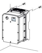
3 Mount the VFD on the wall or inside a panel using the two upper bolts, and then fully tighten the mounting bolts. Ensure that the VFD is placed flat on the mounting surface, and that the installation surface can securely support the weight of the VFD.
