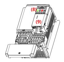
■ Install the front cover (10) and installation is completed.
