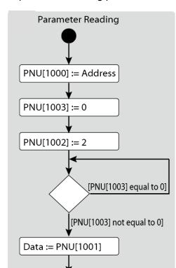
The following diagram explains the parameter reading procedure.
