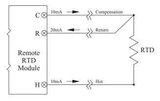
The connection wire from the Remote RTD Module to the RTD will typically have all three conductors the same size and length. This means that the resistance of each conductor will be the same. Call the resistance of each conductor  $R_{lead}$ .
