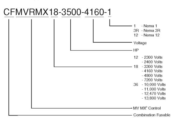
Example of Model Number: CFMVRMX18-3500-4160-1 A Combination Fusable RediStart starter with MV MX<sup>3</sup> control, 4160 Volts, 3500 Horse Power, NEMA 1 Enclosure.
