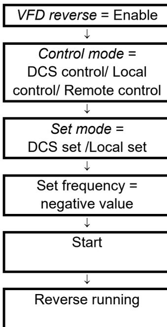
For analog reference or switch reference, set *Control mode* to 'Remote control' and *Remote start/stop mode* to 'Level mode'. You can then control the motor to start and stop in reverse through the level reverse start/stop signal terminal on the interface board.
