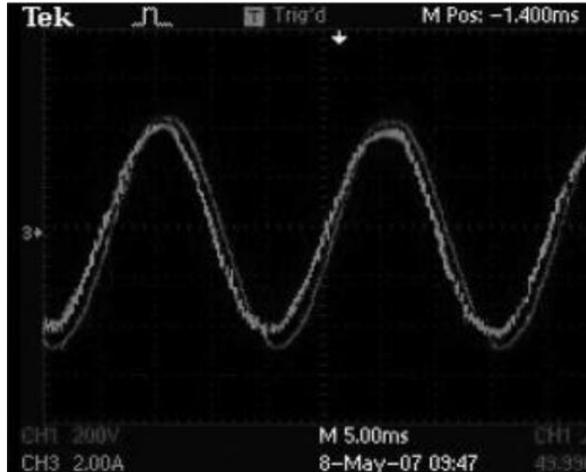
The MV VFD uses power cells in a series connection using H-bridge multilevel overlapping PWM technology. This provides for an output waveform with low harmonic content and a nearly perfect sine wave (see *Output line voltage waveform* on page 12 and *Output current waveforms* on page 13). Compared with other forms of medium voltage large-capacity VFDs, our MV VFD has the following advantages:
