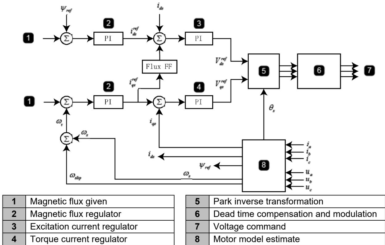
The VFD uses the motor model, measured stator voltage  $u_a, u_b, u_c$  and stator current  $i_a, i_b, i_c$  to calculate magnetic flux  $\Psi_{ref}$ , synchronous speed  $\omega_s$ , synchronous electrical angle  $\theta_s$  and slip  $\omega_{slip}$ .
