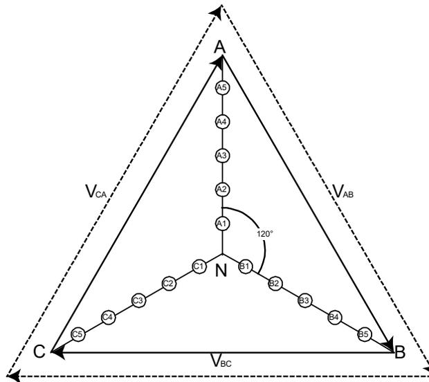
If one power cell fails and is bypassed, the output voltage becomes unbalanced (see *Phase angles for 5-stage VFD, one power cell bypassed*)
