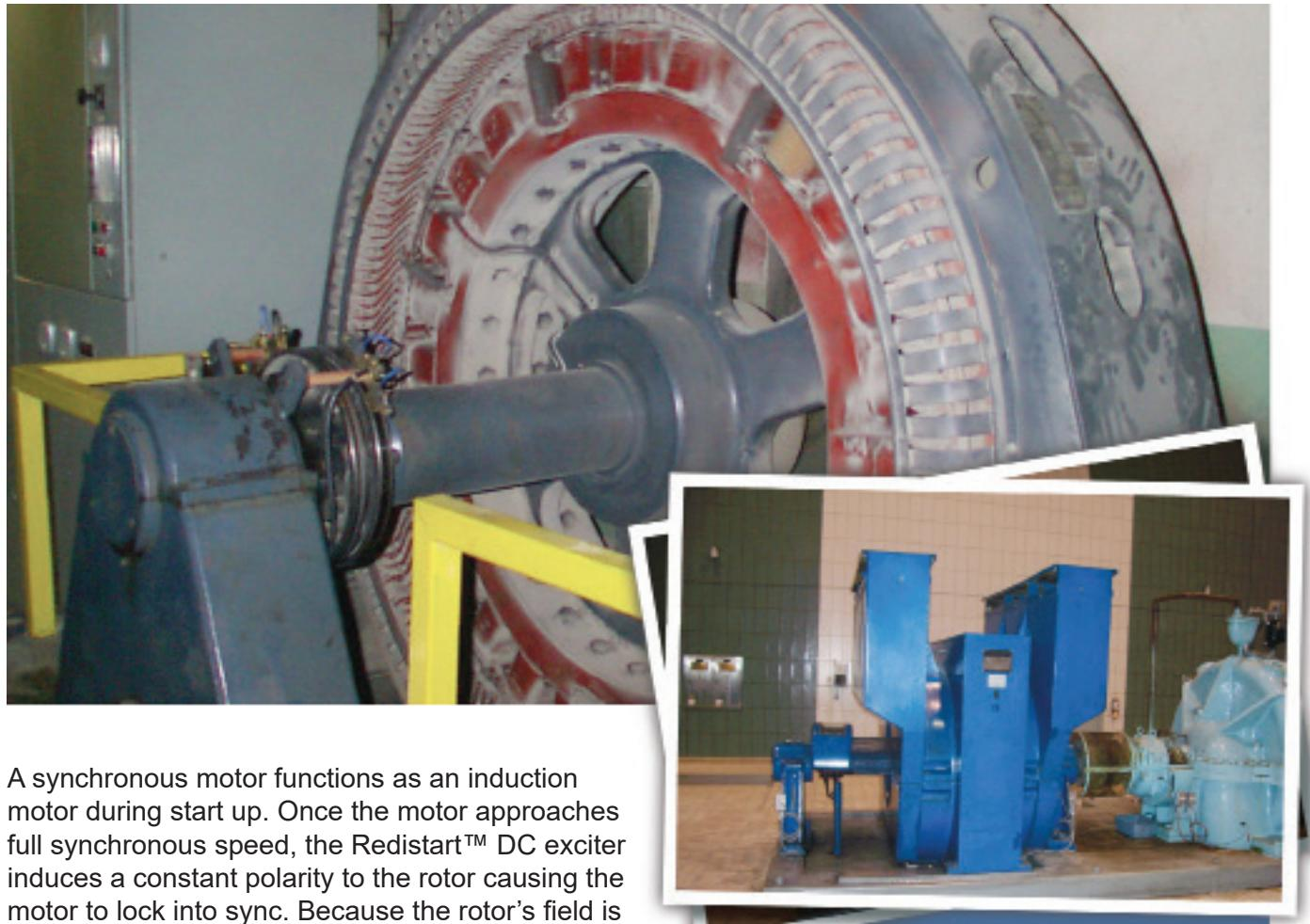
A synchronous motor functions as an induction motor during start up. Once the motor approaches full synchronous speed, the Redistart™ DC exciter induces a constant polarity to the rotor causing the motor to lock into sync. Because the rotor's field is constant and separately excited, there is no slip required to produce torque. This allows the motor to run at synchronous speed.
