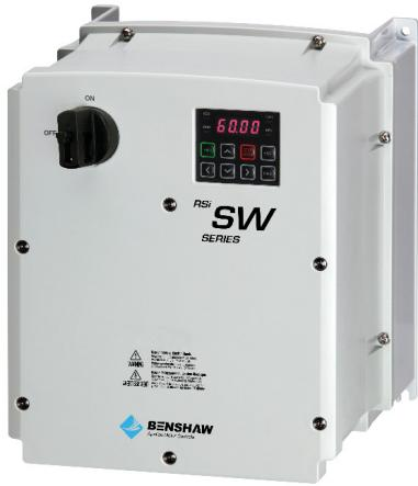
Benshaw SW Series NEMA 4X Washdown Drives are heavy duty rated for applications from 0.5-30HP. Designed for high pressure washdown, all SW Series drives feature a rugged UL Type 4X (IP66) indoor rated polycarbonate enclosure that exceeds NEMA 1, 12, 4 and 4X standard. A convenient built-in power disconnect switch, 4 digit- 7 segment display and optional remote keypad make it easy to control.
