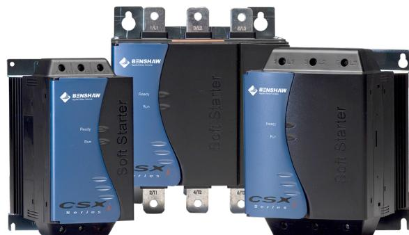
Benshaw CSXi Series Low Voltage Soft Starters are compact, easy-to-use soft starters with built-in motor protection. CSXi Series Low Voltage Soft Starters provide greater control for starting and stopping of three phase motors, and, most models only 6.5 inches (165mm) deep, Benshaw's CSXi Series starters are easy to mount in shallow enclosures.
