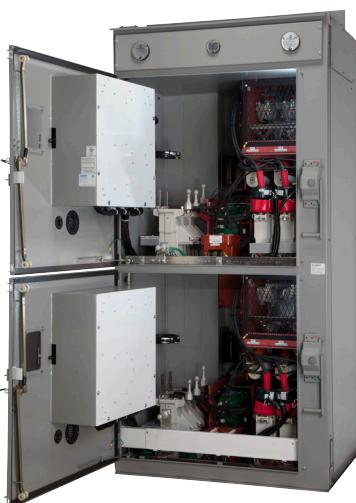
Benshaw's MVDH Two-High Starters provide separate medium and low voltage sections for each starter. Both sections include a complete starter - load break disconnect switch, Class R rated fuses, inline and bypass contactors and to allow complete independent control of two motors. Solid state starting option is available.
