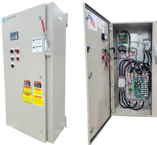
The RX2E / RX3E Enclosed Combination Soft Starter is a rugged, simple to use soft starter with built-in motor protection, providing greater control in starting and stopping of three phase motors. RX2E / RX3E Series Enclosed Combination Soft Starters come standard with a circuit breaker, full voltage rated emergency bypass contactor, door mounted Start/Stop push buttons, Local/Off/Remote selector switch and door mounted keypad.
