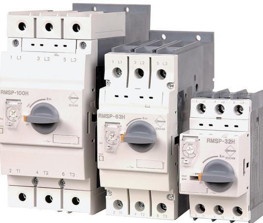
RMXP Series manual starters offer efficient motor starting functionality in a compact design. Protection functions include circuit, motor, starter and phase failure protection. They couple directly to RC Series contactors for a complete electro-mechanical combination starter.
