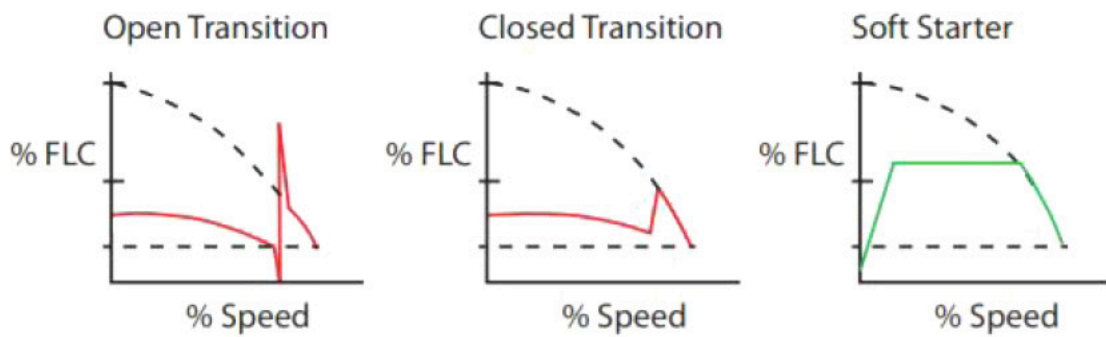
Figure 6. A graphical representation of the current and speed relationships between the various methods.
