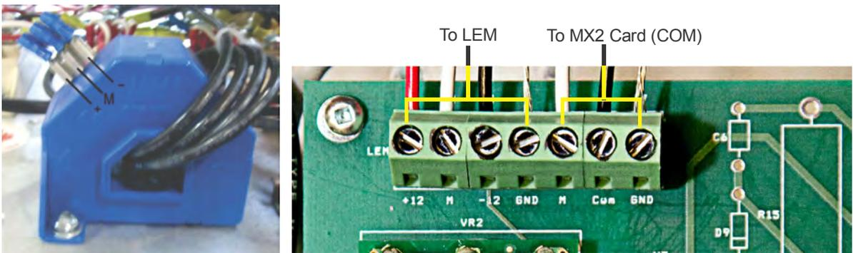
Figure 21: Hall Effect Connections (0 - 700 Amps)
