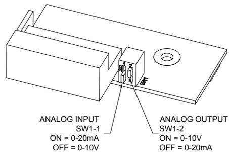
The terminals for the Analog input on the MX2 card (TB5) are as follows:
