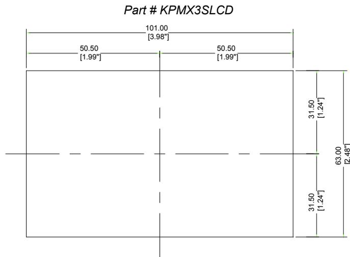
Figure 13: Large Display Keypad Mounting Dimensions
