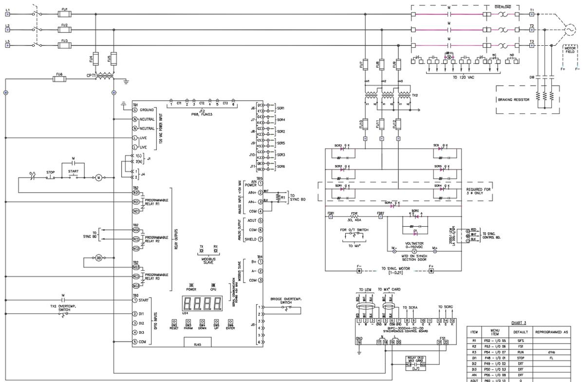
The dynamic braking resistor is sized to 3X the motor FLA at rated motor voltage. For example, motor with stator rated 600VAC, 380A, rated 2 starts/hour hot.
