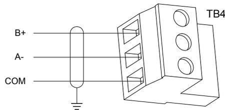
Figure 26: Modbus Network Wiring Example
