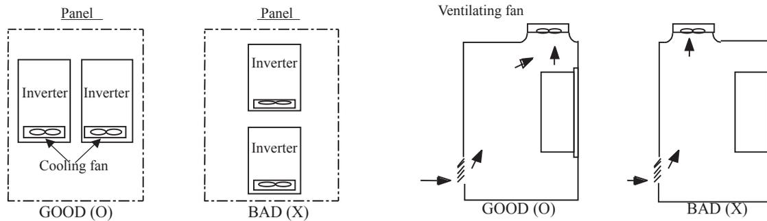
[When installing several drives in a panel]
