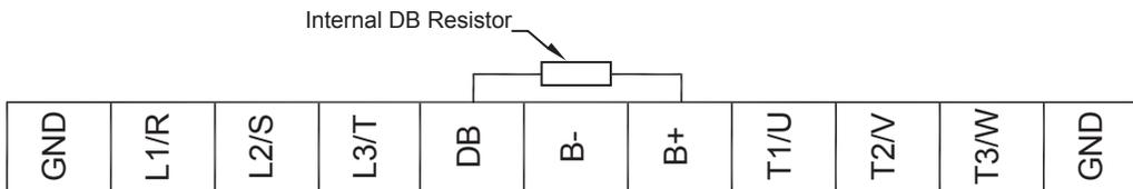
Figure 12: RSi S4 Power Terminals: Frame 4 and 5
