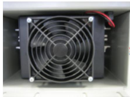
You must now disconnect the fan wires (B, R) from the J1 terminals. Frame 2 will have fan wires (B and R) connected to the J1 and J9 terminals. There is a grommet that the wires travel through to get to the J1 and J9 terminals. This grommet must be loosened so the wires can get out. After installing new fans, this grommet must be tightened.
