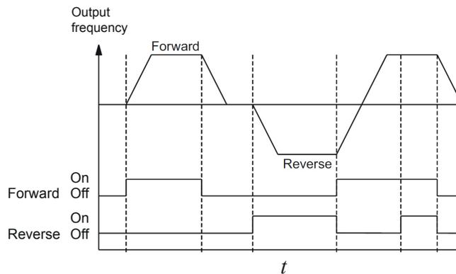
⚠ **NOTE:** That in the above diagram, when both forward and reverse are on (closed), the drive runs forward. This is the case whenever both FWD and REV are closed at the same time.
