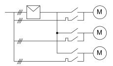
• the soft starter must be suitably rated for the total start duty
